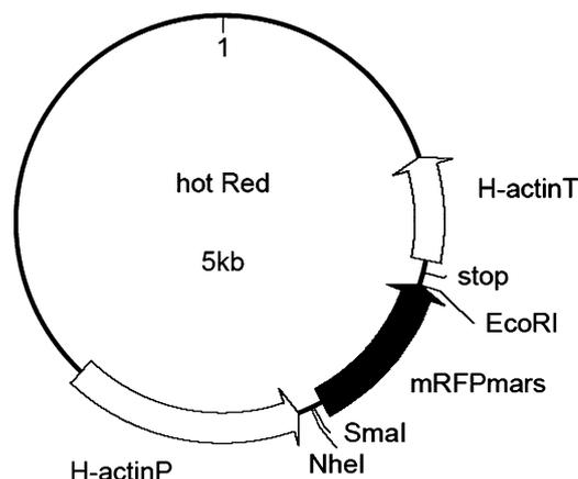
**Fig. 1.** Vector map for hot Red. The *Hydra* actin promoter (H-actinP) directs strong expression of fusion proteins. The fragment of the sequence can be cloned into the vector either at the N- or at the C-terminus of mRFPmars.
